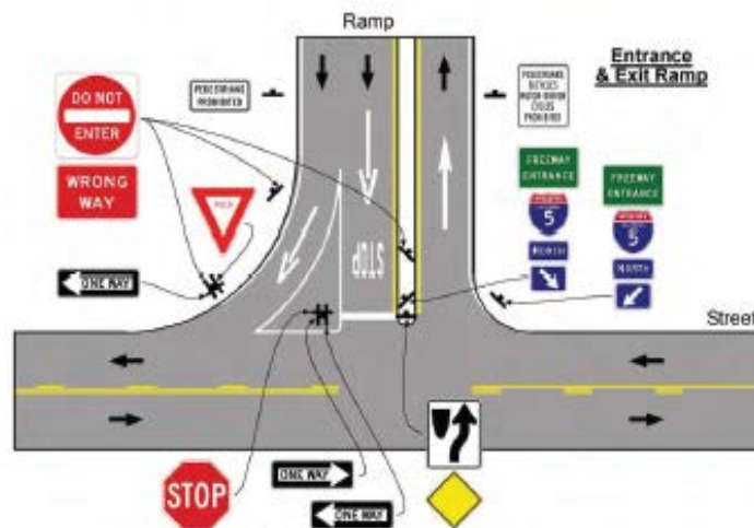
Figure 2.4. Standard signing and marking layout in California (Cooner, Cothron, and Ranft 2004).
